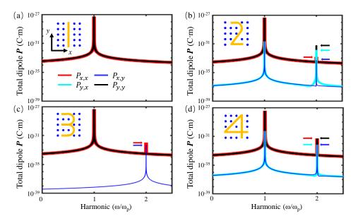
**Fig. 4.** Nano-QR-codes. Harmonic generation in a square nanoparticle with different atomic defect patterns. (a)-(d) Frequency dependence of the electric dipole moment of a square particle (insert) with defect patterns (a) "1", (b) "2", (c) "3", (d) "4" in response to optical pumping at frequency  $\omega_p$ .  $P_{\alpha,\beta}$  indicates the  $\alpha$ -component of the particle's electric dipole moment caused by  $\beta$ -polarized pumping.
