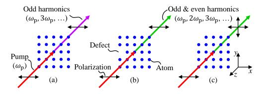
**Fig. 1.** Defect-induced optical nonlinearity. (a) Along the optical axis, as shown, a square particle will only generate odd harmonics of the pump frequency  $\omega_p$  without polarization change. The presence of defects enables even harmonic generation (b) without and (c) with polarization change.
